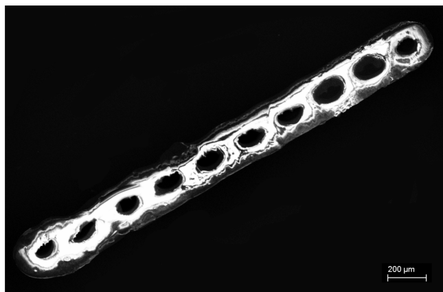
Figure 1. Scanning electron micrograph showing a side view of the FEP MCFs. The image was taken at 171 \times magnification. The average hydraulic diameter of each capillary is 104.2 \mu\text{m} \pm 10.6 \mu\text{m} with an average wall thickness of 61.5 \mu\text{m} \pm 17.1 \mu\text{m} .
